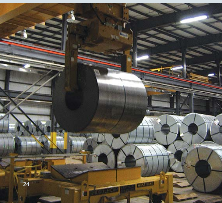
A crane lifts a coil to be stacked in the warehouse
