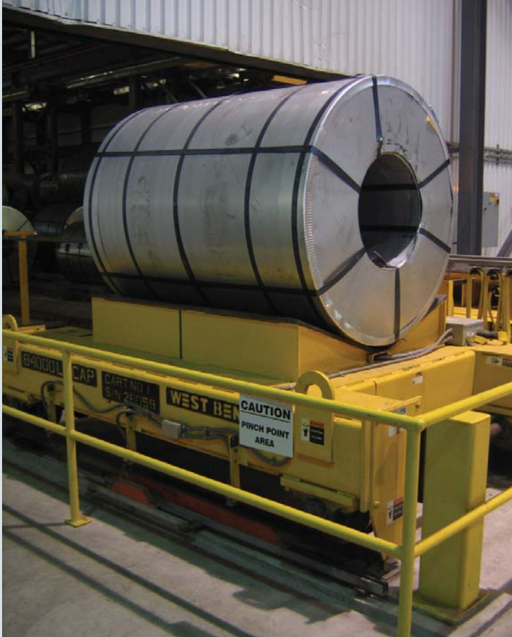
An automated transfer cart shunts a steel coil into the warehouse
